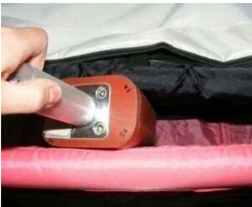
Picture 9: Head entrapment was observed
