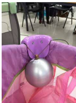
Picture 5: Failure for snagging points
