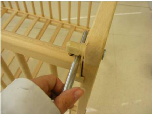
Picture 1: Showing potential finger entrapment
