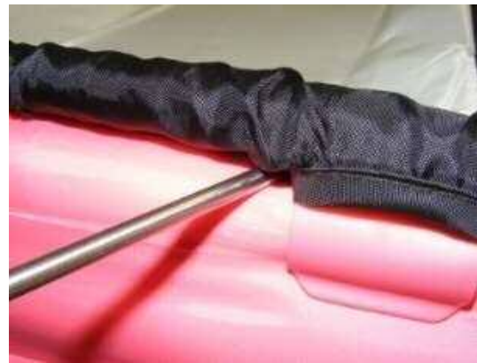
Picture 10: Finger crushing hazard
