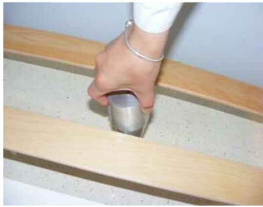
Picture 2: Showing potential limb entrapment
