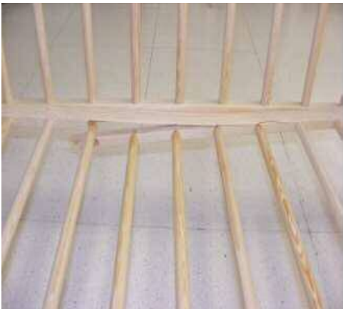
Picture 3: Poor construction - failure of slats in cot base
