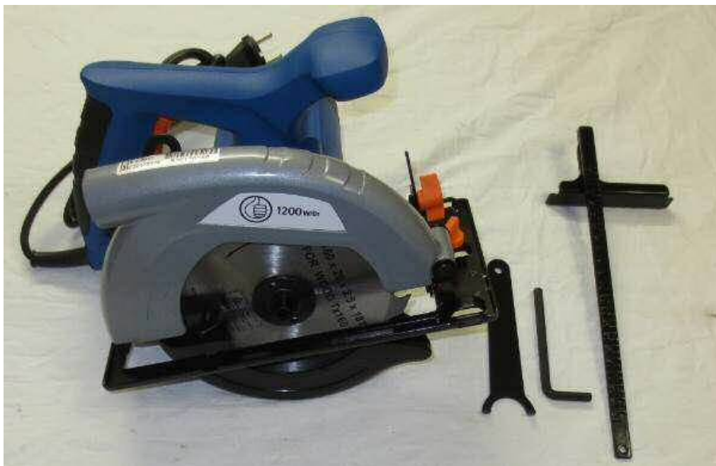
Figure 4: Example of a handheld electrical circular saw in the cheaper price classes with accessories.
