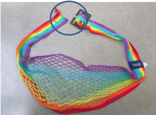
Picture 7: Failure for 8.5 Durability The carrier breaks
