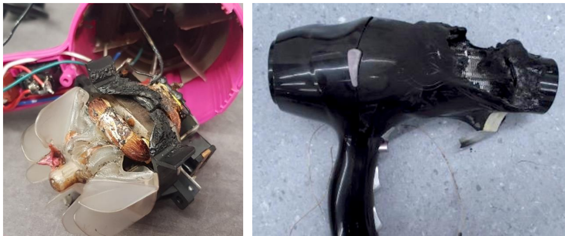
Figure 11 Motor winding overheating and no protection against stalled motor
