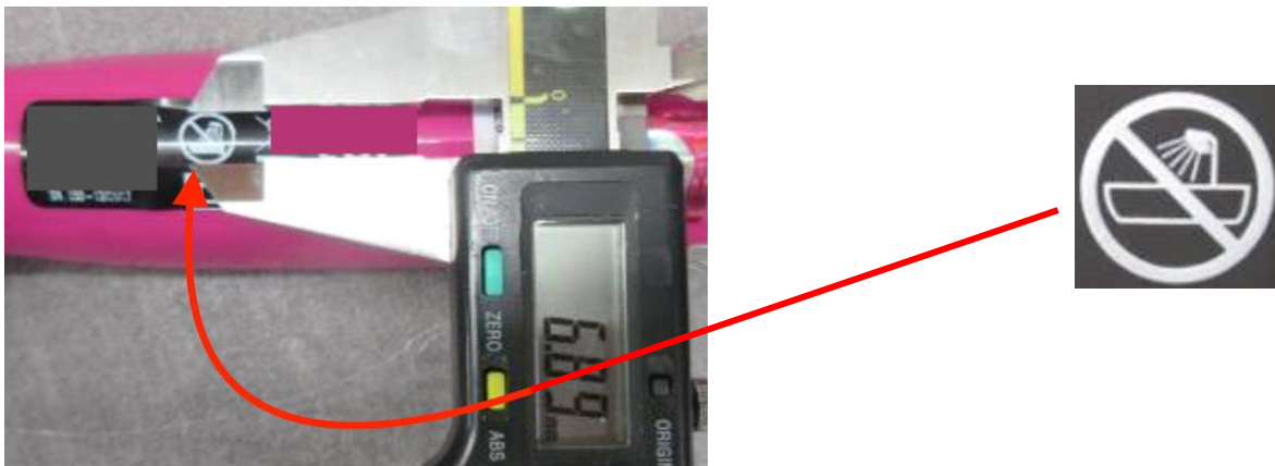
Figure 8 Undersized warning symbol
