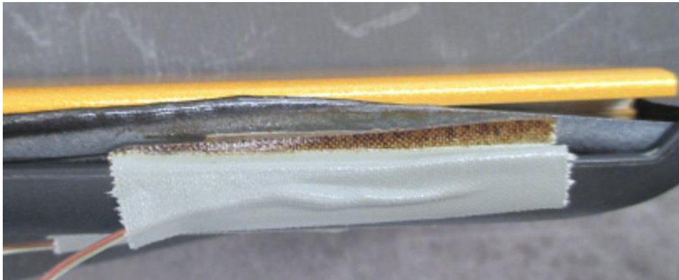
Figure 14 Enclosure deformation after abnormal operation test
