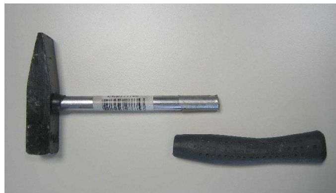
Figure 9 - RAPEX notification no. 0125/06 deals with a hammer where the handle breaks.
