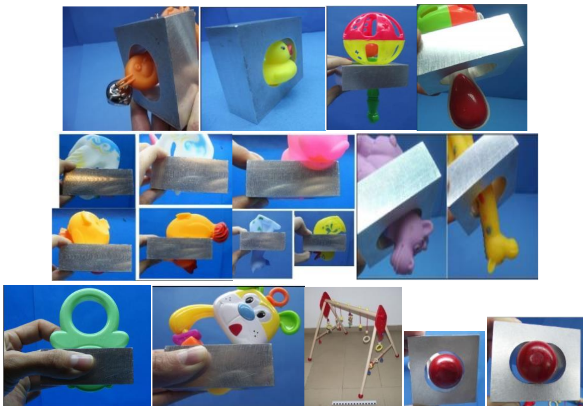
Figure 26. Detail of samples non-complying with clause 5.8
