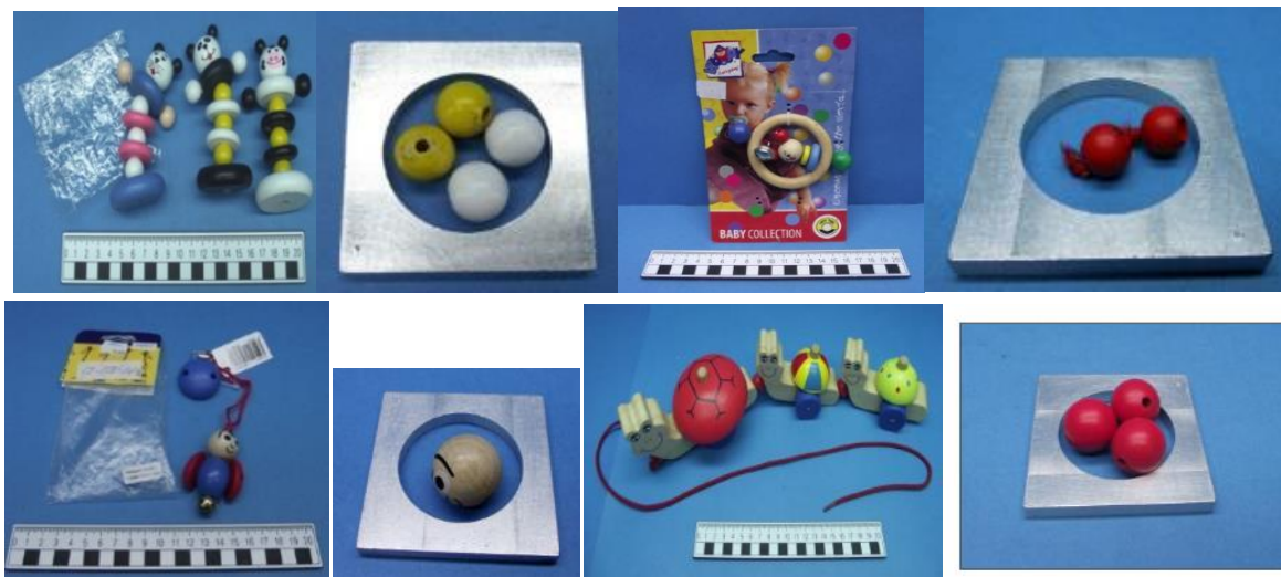
Figure 29. Detail of samples non-complying with clause 5.10 after tension tests
