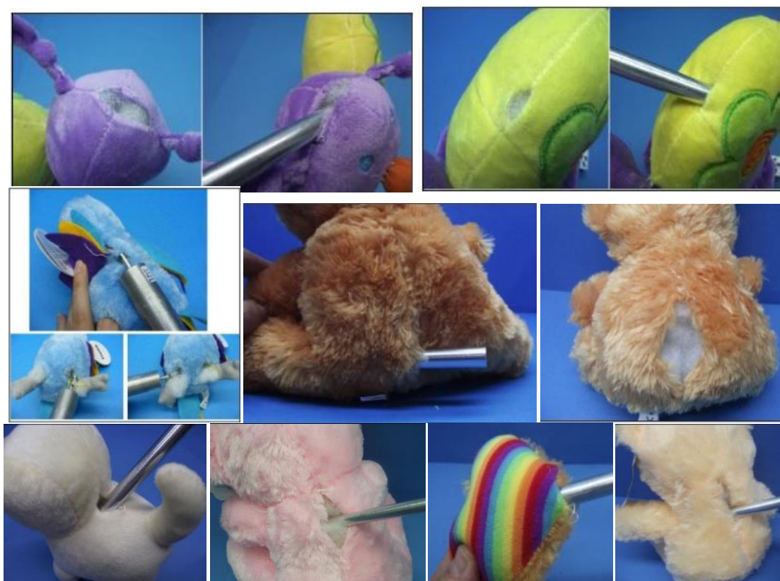
Figure 22 Detail of samples non-complying with clause 5.2
