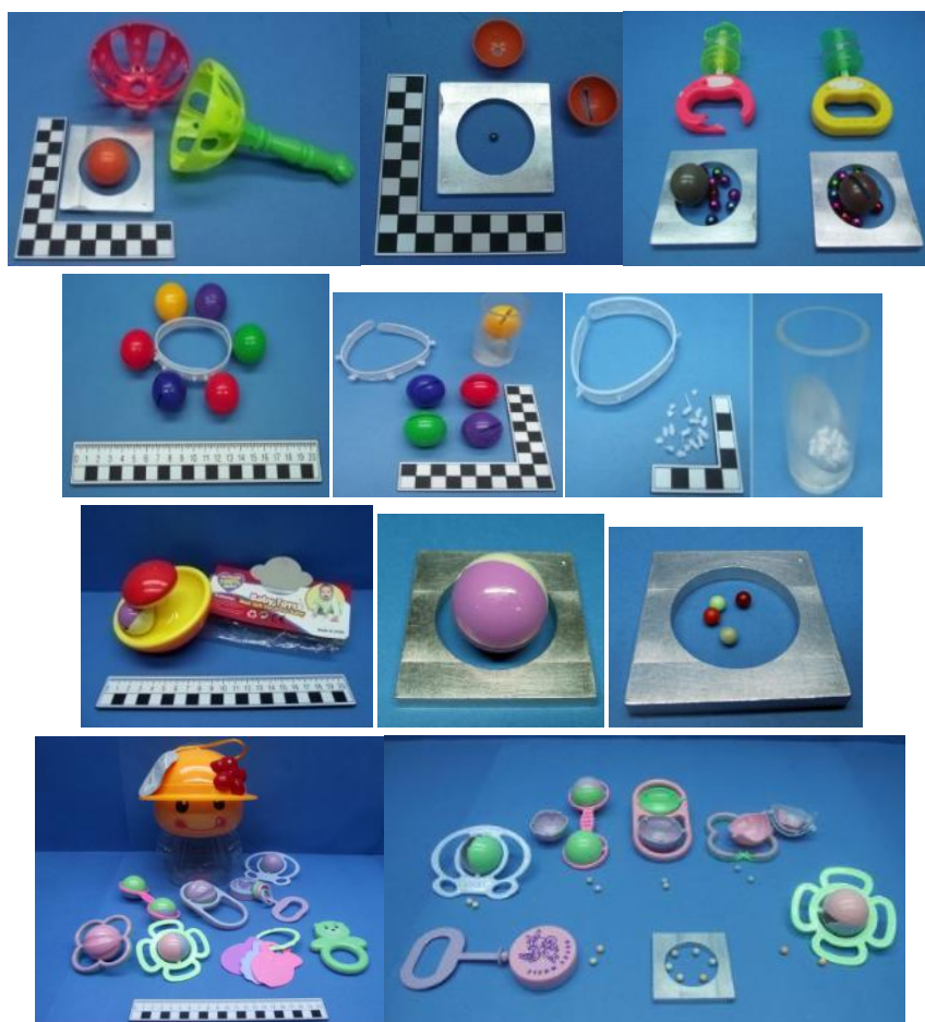
Figure 28. Examples of samples non-complying with clause 5.10.
