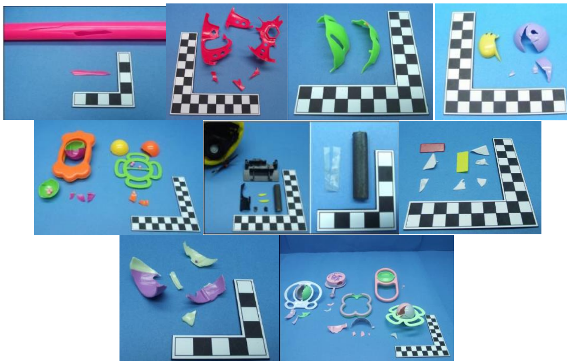
Figure 9. Sharp points after 8.7 Impact test
