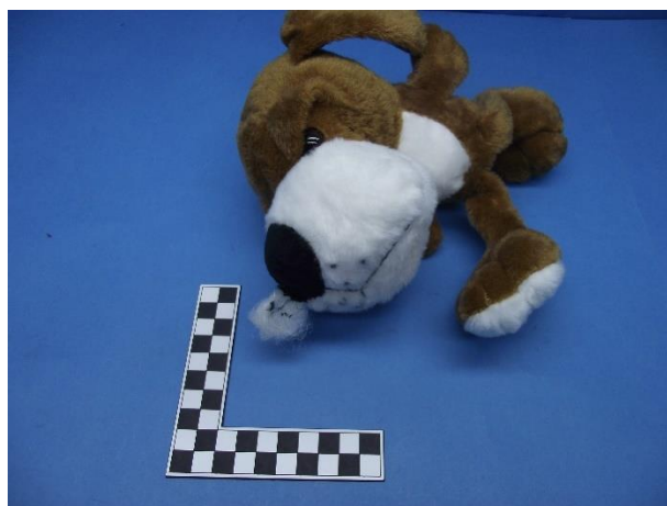
Figure 21 Sample with open seam & fibrous filling material easily accessible
