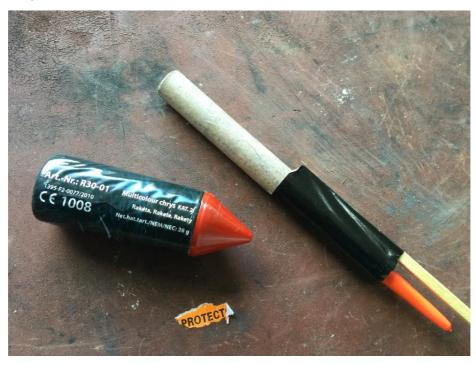
Figure 9 - Rocket in which the plastic fuse cover precluded access to the fuse and in which the head of the rocket became detached when the lab staff attempted to remove the fuse cover.
