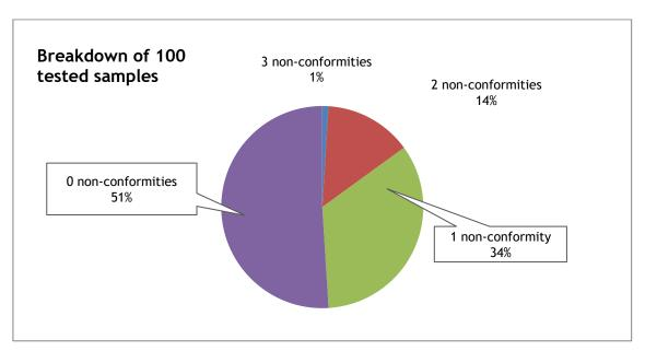
Figure 7: The share of saws that passed all tests, failed to comply with one clause, two clauses and three clauses.
