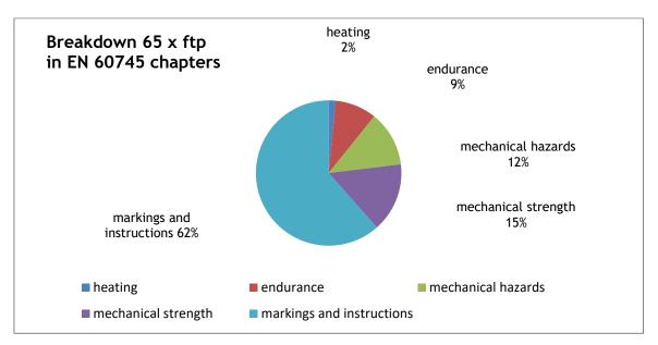
Figure 6: Overview of non-compliances identified in the 100 samples regarding safety requirements from EN 60745.
