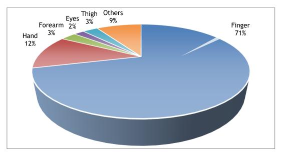
Figure 2: Inflicted body part in accidents with circular saw (based on 481 accidents in 2012-2014)
