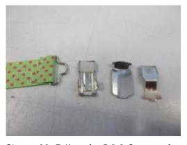
Picture 20: Failure for 5.2.2 Garment fastener test fastener
