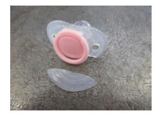
Picture 2: Failure for 9.1.2 Impact test The shield broke and small parts were generated
