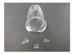
Picture 7: Failure for 11.7 Impact resistance
