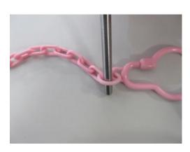
Picture 19: Failure for 5.1.4.1 Finger entrapment
