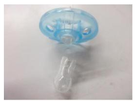
Picture 3: Failure for 9.3.2.1 Tear Resistance of teat
