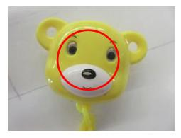
Picture 13: Failure to 5.1.4.1 Ventilation (un-ventilated area exceeding 25mm)
