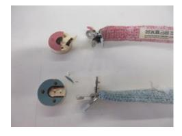
Picture 21: Failure for 5.2.3 Tensile
