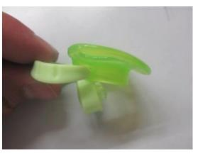
Picture 4: Failure for 9.4.2 Knob, plug and/or cover retention
