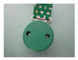
Picture 12: Failure to 5.1.4.1 Ventilation (ventilation holes are too small)
