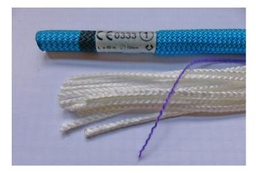
Figure 7 - Structure of a dynamic single climbing rope and marking band Credit.: Laboratory
