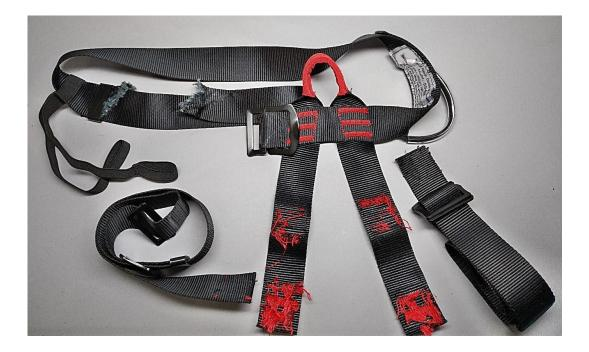
Figure 19 - Harness torn during the harness strength test (Photo.: Laboratory)
