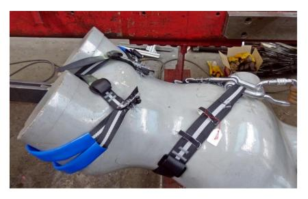
Figure 20 - Failure of safety stitching during the harness strength test (Photo: Laboratory)
