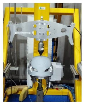
Figure 12 - (Left) Energy absorption capacity test - (Right) Penetration resistance test (Photo.: I. Fraser)
