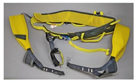
Figure 21 - Harness torn during the harness strength test (Photo: Laboratory)
