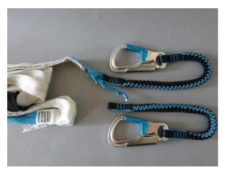
Figure 22 - Breakage of the secure resting connection of an EAS during the static test (Photo: Laboratory)
