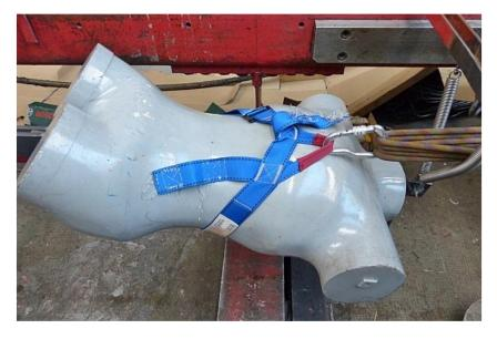
Figure 17 - Harness torn during the harness strength test (Photo: Laboratory)
