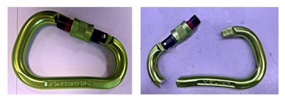
Figure 10 - Basic connector before and after a strength test (Photo: Laboratory)
