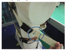
Picture 7: Failure for 8.5 Durability The carrier breaks
