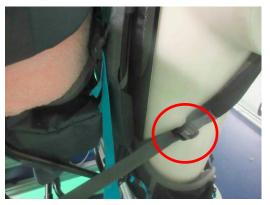
Picture 2: Failure for 6.4 Cords The cord is longer than 220mm
