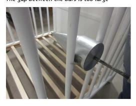
Picture 12: Failure for 4.4.3 Head entrapment on the outside The child's head could become stuck
