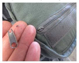
Picture 3: Failure for 6.8 Carer attachment
