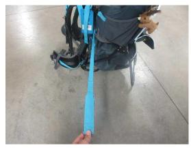
Picture 4: Failure for 6.9 Dynamic systems strength The strap broke
