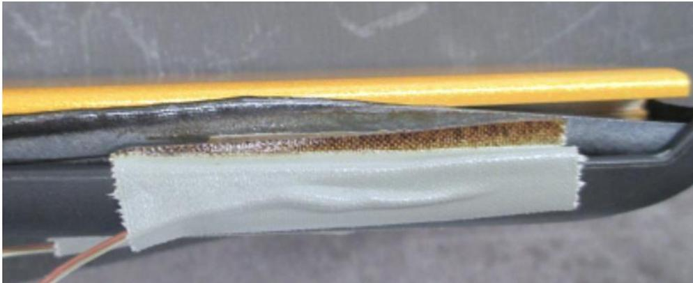
The hair straighteners, as tested, are class II appliances where protection against electric shock does not rely on basic insulation<sup>6</sup> alone. Additional safety precautions are necessary, such as double or reinforced insulation. During these abnormal operation tests the electrical insulation is subjected to a high voltage to determine its overall electric strength. **All three samples failed the electric strength test.**
