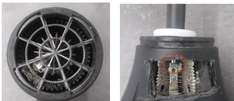
Clause 19 of the standard deals with abnormal operation where “(...) appliances shall be constructed so that as a result of abnormal or careless operation, the risk of fire, mechanical damage impairing safety or protection against electric shock is obviated as far as is practicable”.
