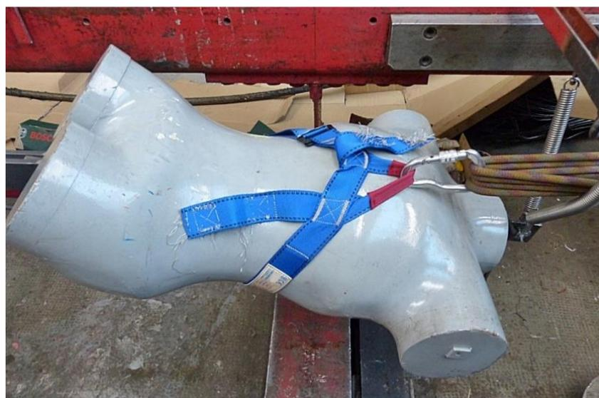
**Figure 17 - Harness torn during the harness strength test**
