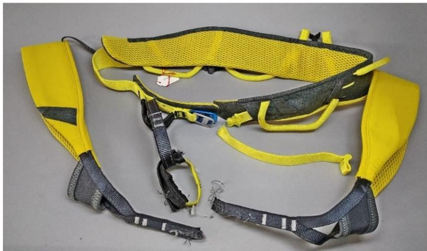
**Figure 21 - Harness torn during the harness strength test**
