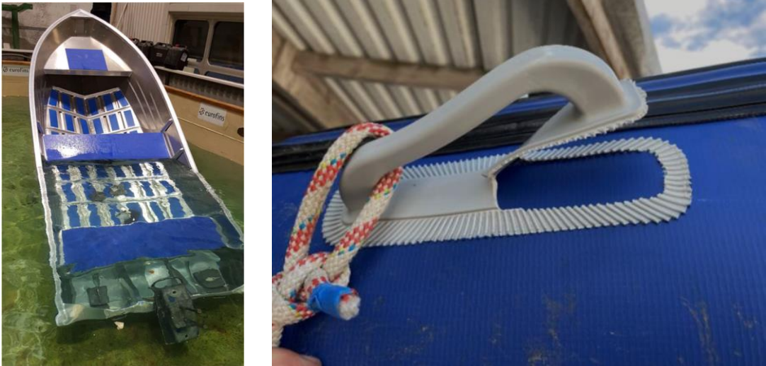
Figure 14 - Failure of a rigid hull craft during the level (swamped) flotation test: the aft of the boat is supported by the bottom of the test basin (left); Failure of a grab handle during strength test (right)
