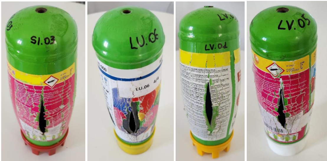
Image 1: Compliant cylinders (without a pressure relief device) after the burst test: the failure was initiated in the cylinder shell, outside the area of the welds
