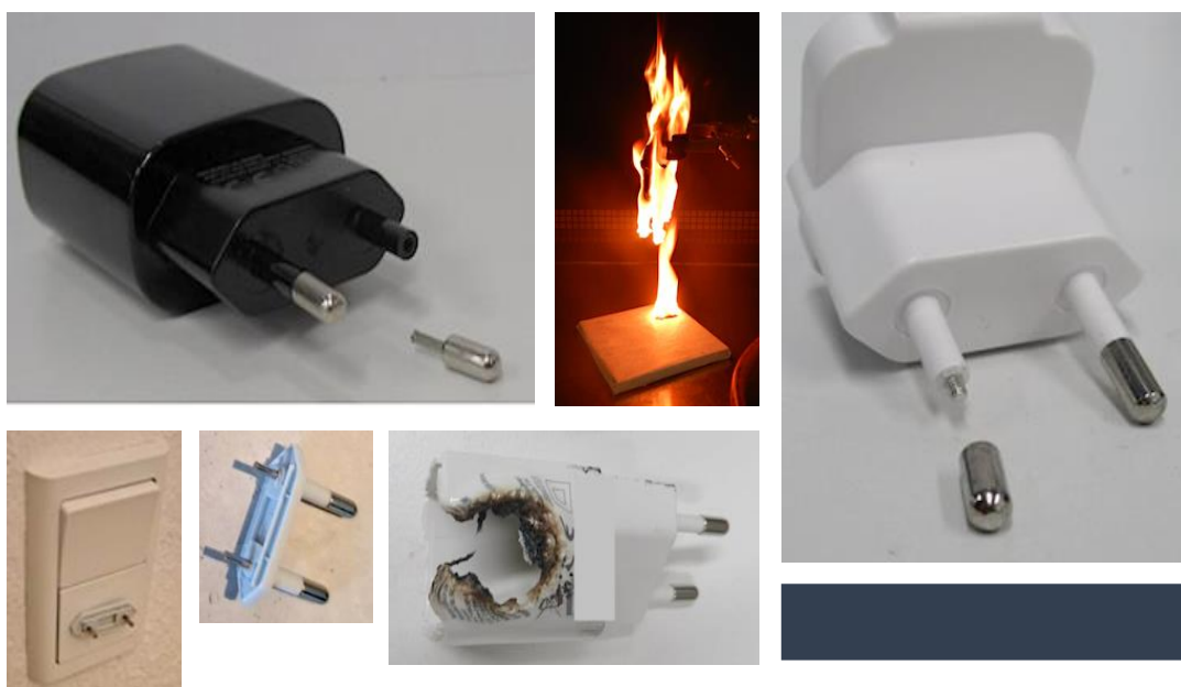
Image 2: Examples of nonconformities detected in the laboratory tests on USB chargers
