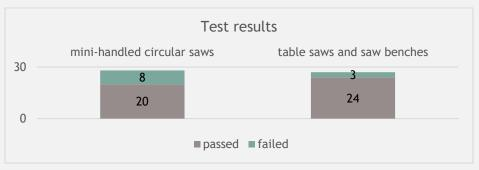
The most serious deficiencies for mini-handled circular saws concerned the lack of endurance of the supply cord and inadequate strength or absence of the base plate.
