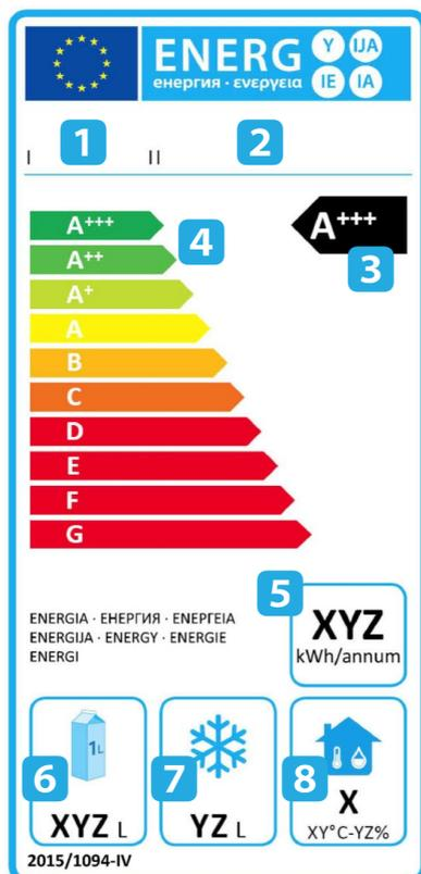
The energy label regulation requires that cabinets are supplied and advertised with an energy label and a fiche from July 2016. From 1 July 2019 the label must show label classes up to A+++<sup>8</sup>. The information items shown on the energy label are explained in the figure below.
