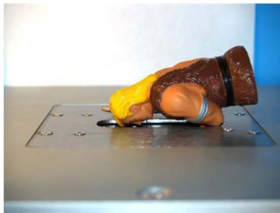
Figure 14. The figure's eyes are smaller than the window opening. Longer sample times may be required on small samples.
