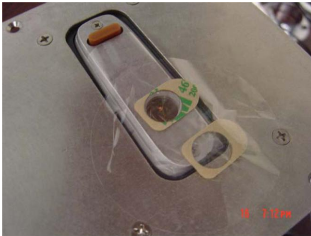
Figure 15. Paint chips secured between two plastic films. One is positioned for analysis.
