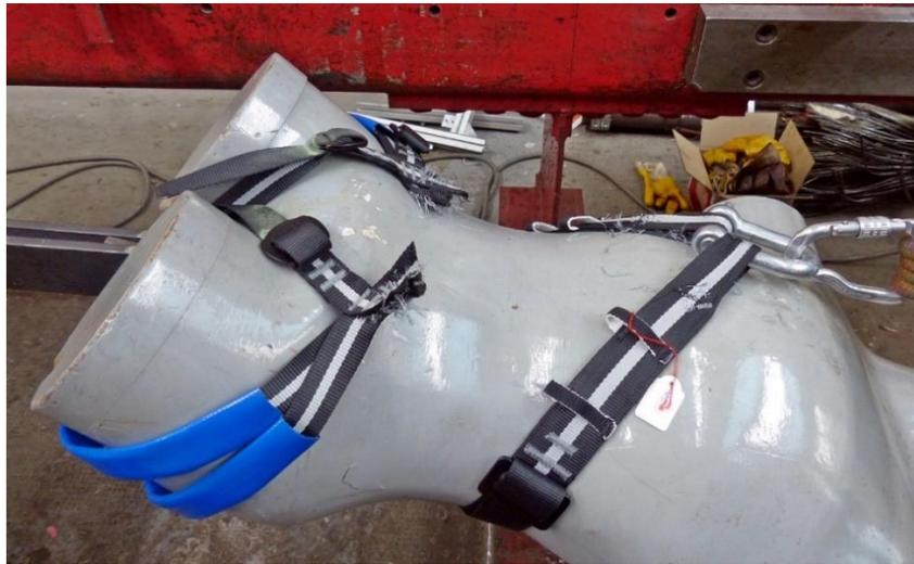
**Figure 20 - Failure of safety stitching during the harness strength test**
