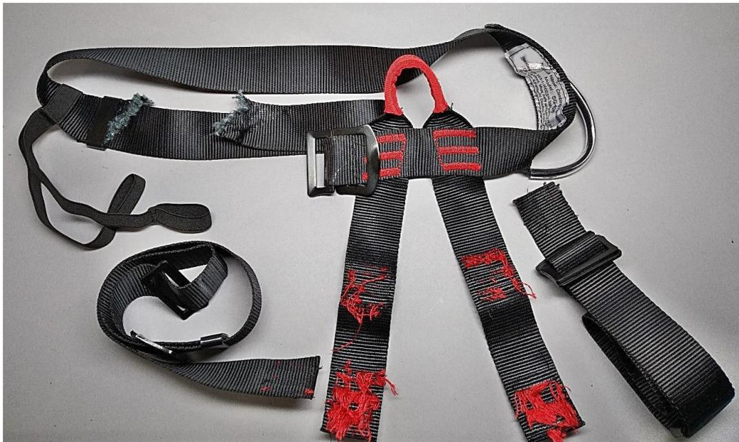
**Figure 19 - Harness torn during the harness strength test**
