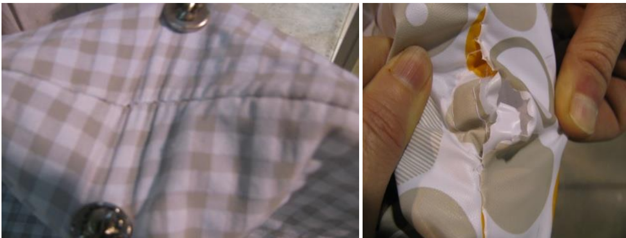
Figure 18 - Example of seams strength test
