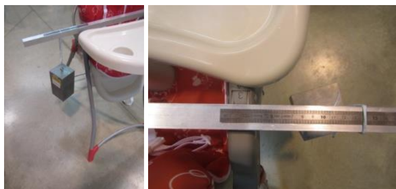
Figure 14 - Sideways stability test
