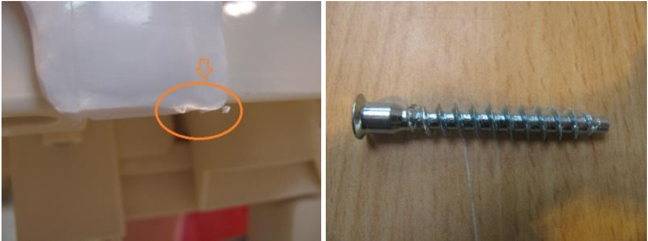
Figure 29 - Examples of burrs, self-tapping screws
