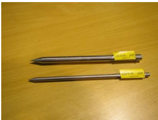
Figure 2 - Gauges used for assessment of finger entrapment
