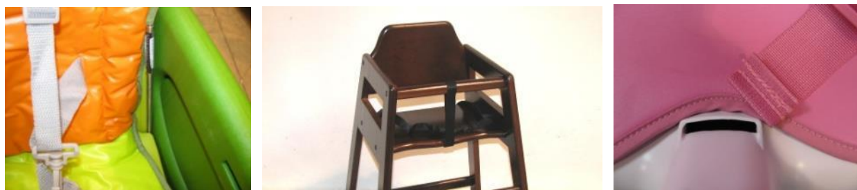
Figure 39 - Examples of active restraint system that did not meet the requirement
