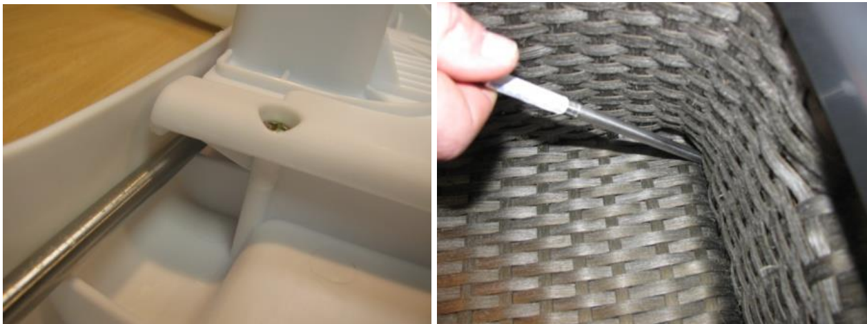
Figure 32 - Examples of openings that create an entrapment: completely bounded, no dimension allows movement of trapped fingers
