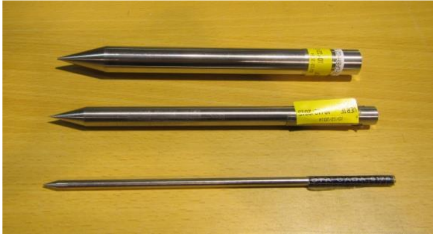
Figure 5 - Gauges for assessment of moving parts
