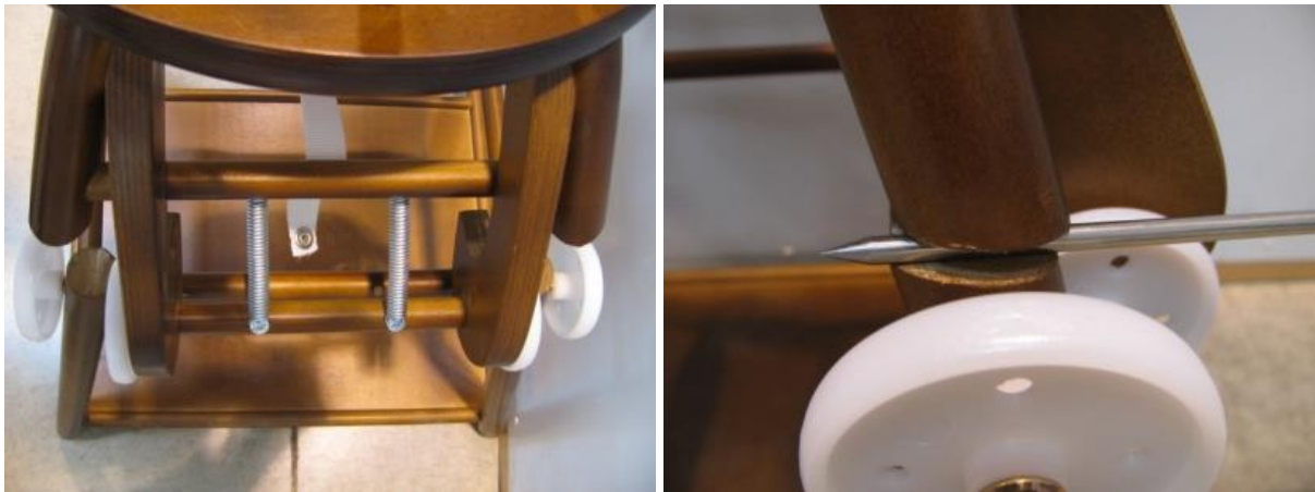
Figure 6 - Example of squeeze point on high chair
