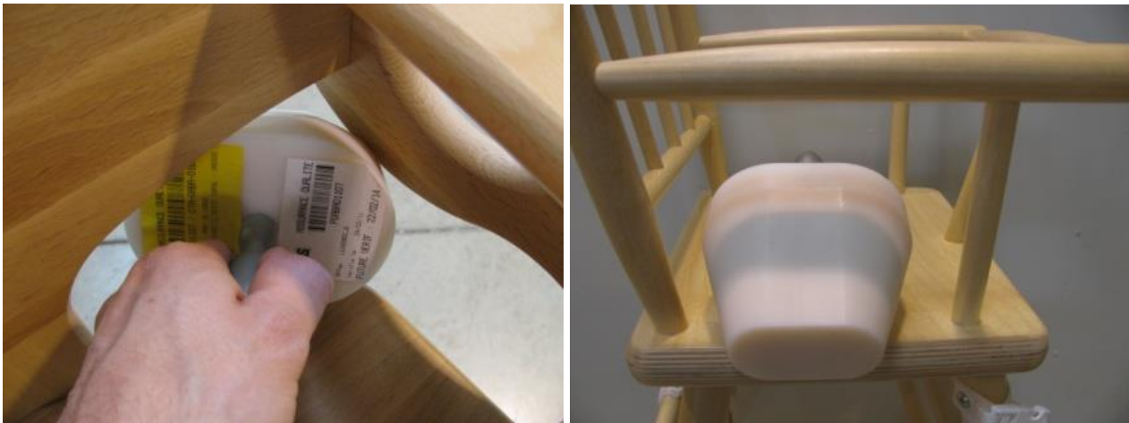
Figure 33 - Example of entrapment of torso
