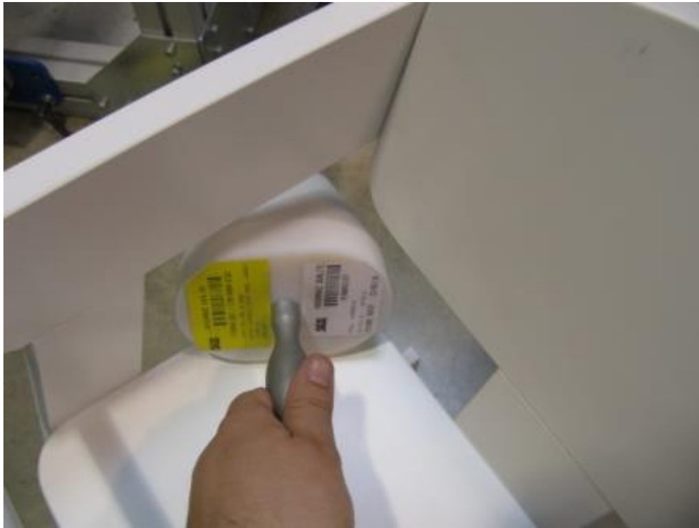
Figure 4 - Example of opening that does not meet the requirement of the standard
