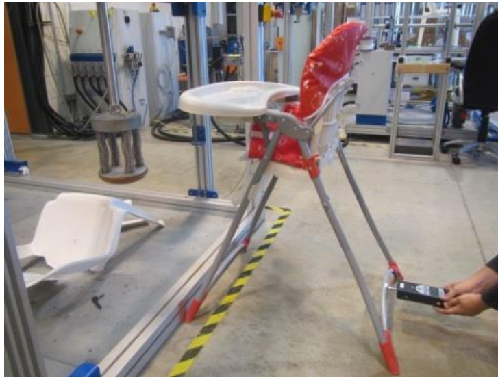
Figure 11 - Locking mechanism strength
