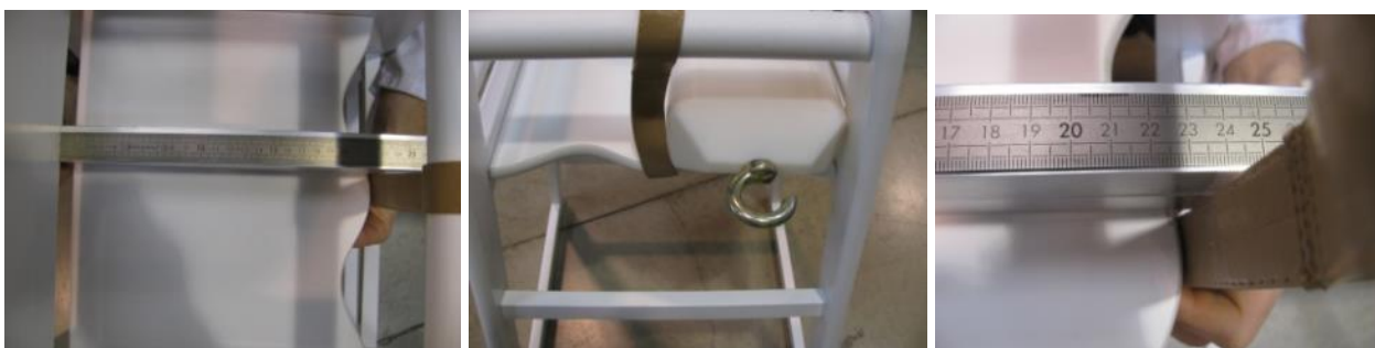
Figure 37 - Example of non-conformities of passive restraint system
