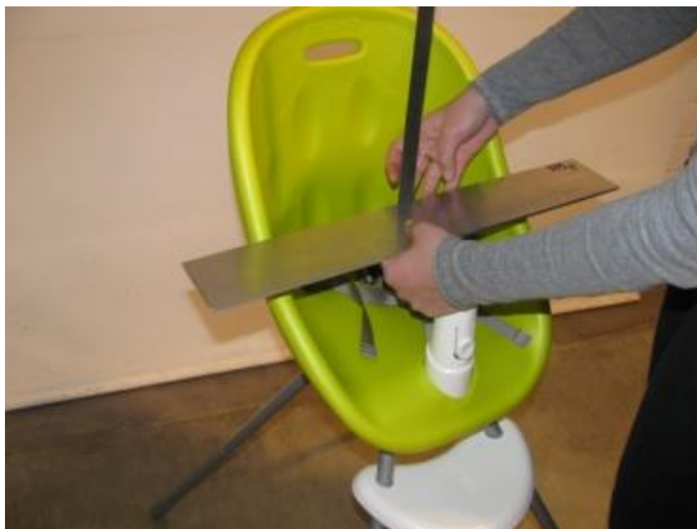
Figure 40 - Example of lateral protections that did not meet the requirement
