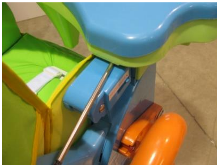
Figure 34 - Example of compression hazard (squeeze point) found between tray and armrest
