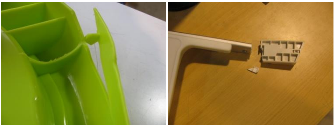
Figure 42 - Example of damage after tray drop test
