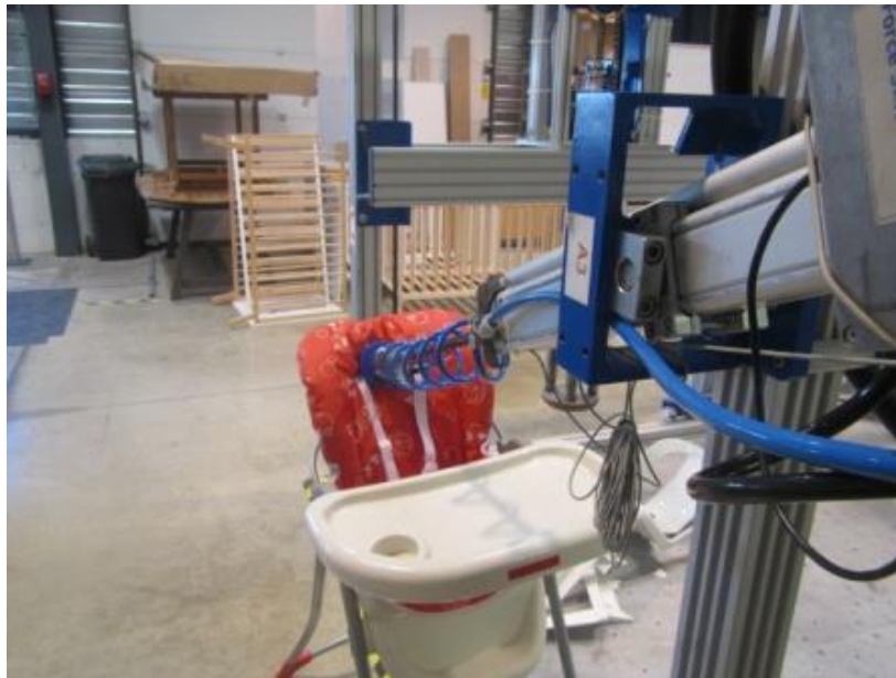
Figure 12 - Strength of reclinable backrest test
