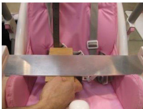
Figure 38 - Example of too low lateral protection
