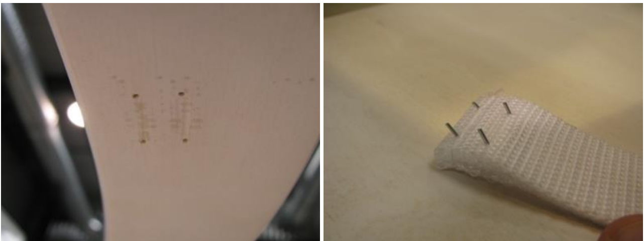
Figure 41 - Example of non-conformity to seat vertical static load test - crotch restraint detached from the horizontal element
