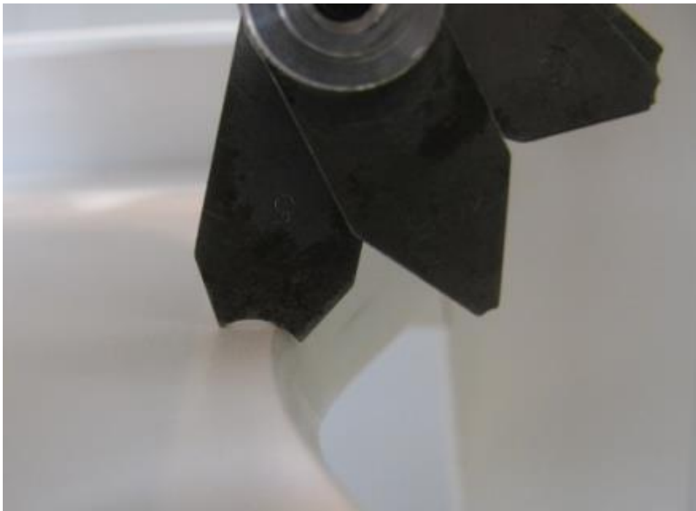
Figure 30 - Example of front edge with a radius < 5 mm
