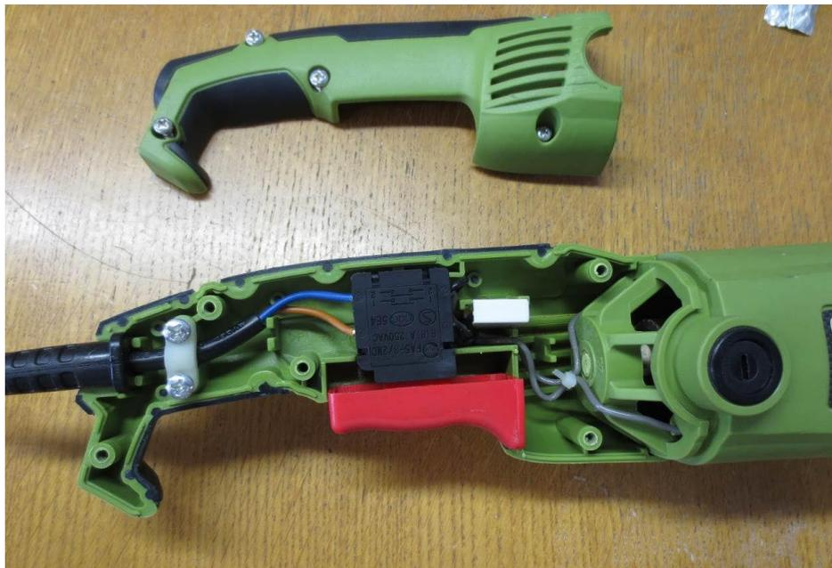
Figure 6: Hold-on grasp category switch with automatic switch off through grasp-release
