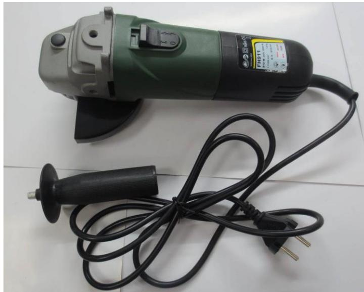
Figure 7: Thump operated lock-on category switch (without restart prevention)
