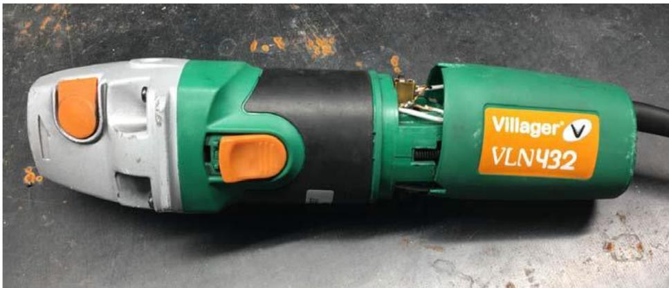
Figure 8: The drop fall test caused a broken housing and discloses life parts
