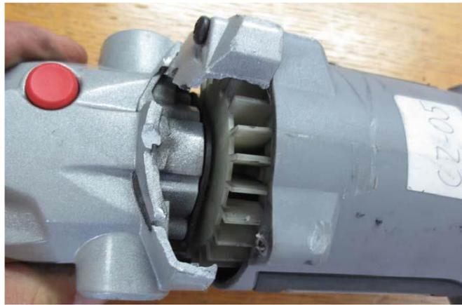
Figure 9: The drop fall test caused a broken housing and discloses rotating parts
