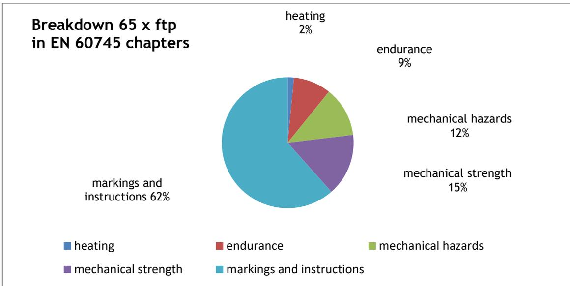
Figure 6: Overview of non-compliances identified in the 100 samples regarding safety requirements from EN 60745.
