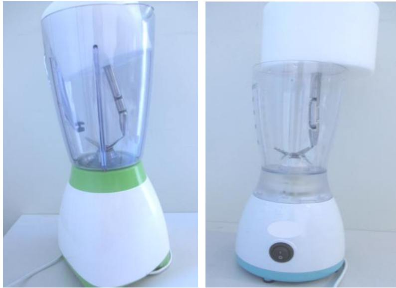
Figure 11 Access to rotating blades with test probe
