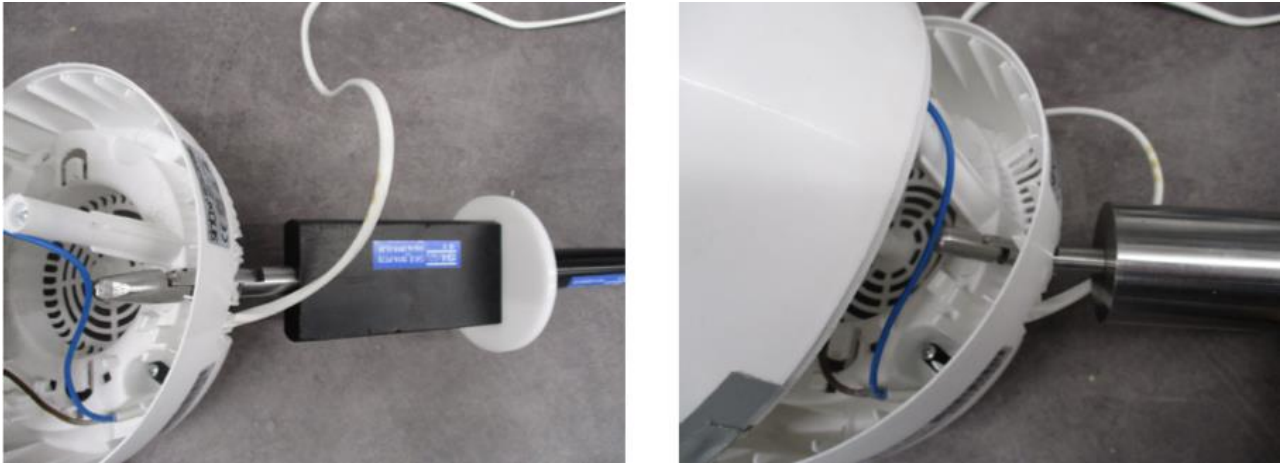
Figure 9 Adult test probe and child test probe access through openings in blender enclosures
