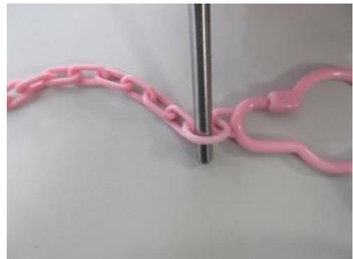
Picture 19: Failure for 5.1.4.1 Finger entrapment
