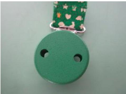
Picture 12: Failure to 5.1.4.1 Ventilation (ventilation holes are too small)
