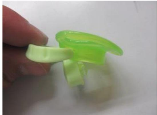
Picture 4: Failure for 9.4.2 Knob, plug and/or cover retention
