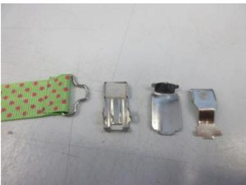
Picture 20: Failure for 5.2.2 Garment fastener test fastener
