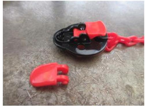
Picture 17: Failure to 5.2.1 Impact
