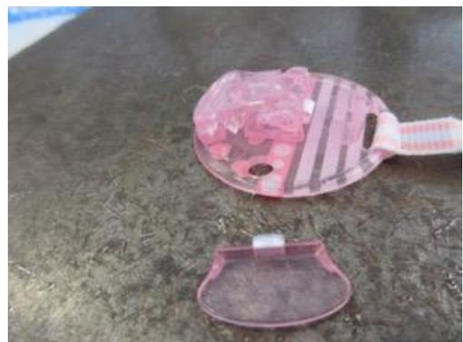
Picture 15: Failure to 5.2.1 Impact
