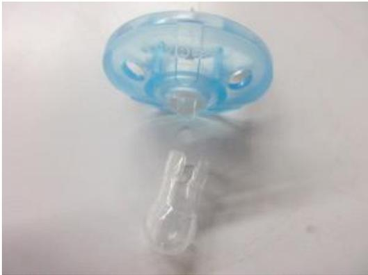
Picture 3: Failure for 9.3.2.1 Tear Resistance of teat
