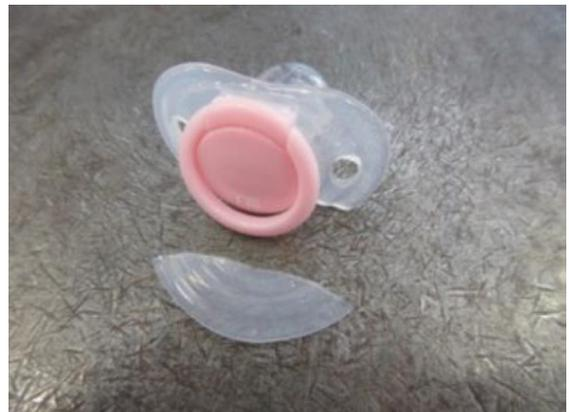
**Picture 2: Failure for 9.1.2 Impact test**
