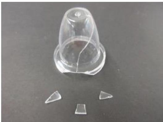
Picture 7: Failure for 11.7 Impact resistance
