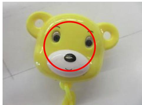
Picture 13: Failure to 5.1.4.1 Ventilation (un-ventilated area exceeding 25mm)
