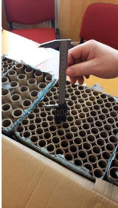
Figure 5 - Sample SL 13 - Compound firework showing that in this part of the firework the tube fired correctly
