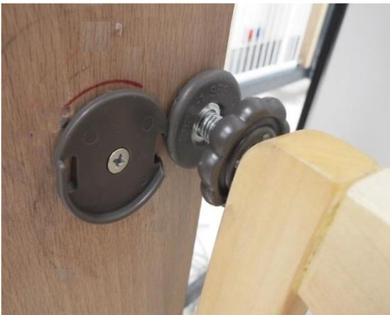
Picture 7: Failure for 6.12 impact test
