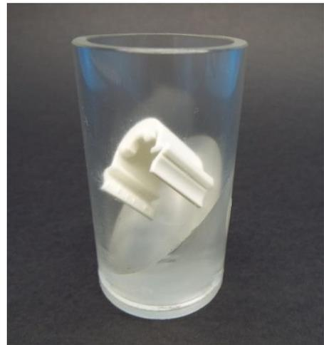
Picture 6: Failure for 6.8 choking hazards
