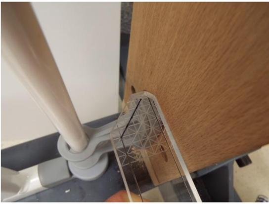
Picture 3: Failure for 6.2 footholds
